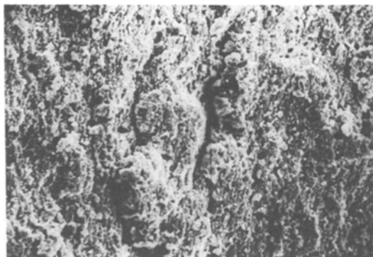
Figure 10 Pitted surface with fissures, sulphur-cured NR, clay-filled ( \times 83 ).
